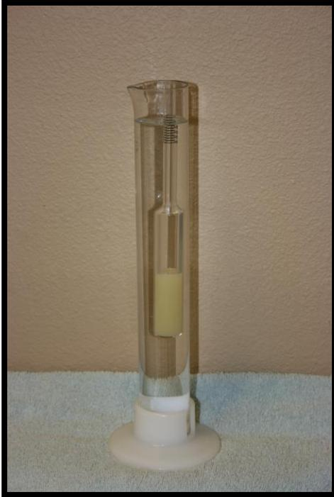
Figure 4. Measuring specific gravity of equine colostrum using a colostrometer.
