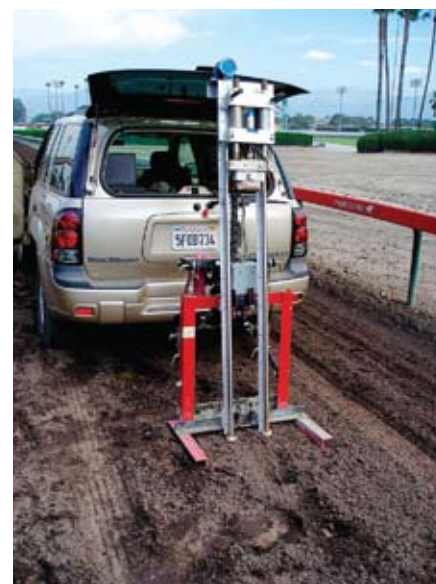
Track Testing Device measures both impact and shear properties of the racetrack.
